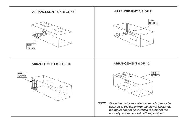
FIGURE 5 - LA300/LB360/LB480 MOTOR ARRANGEMENTS
